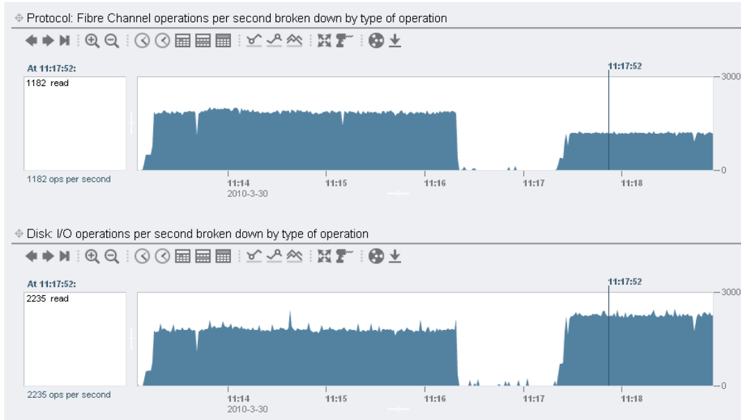
Figure 20. Comparison of 256 and 34 start sectors for EFI labeled LUN
