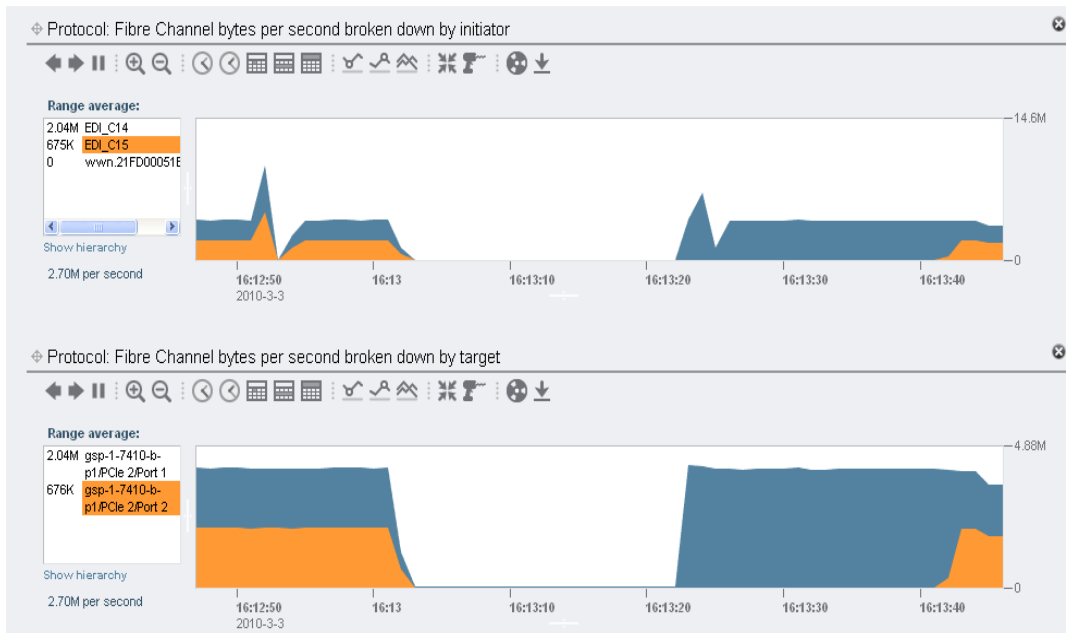
Figure 16. Link disconnected from active Oracle ZFS Storage node
