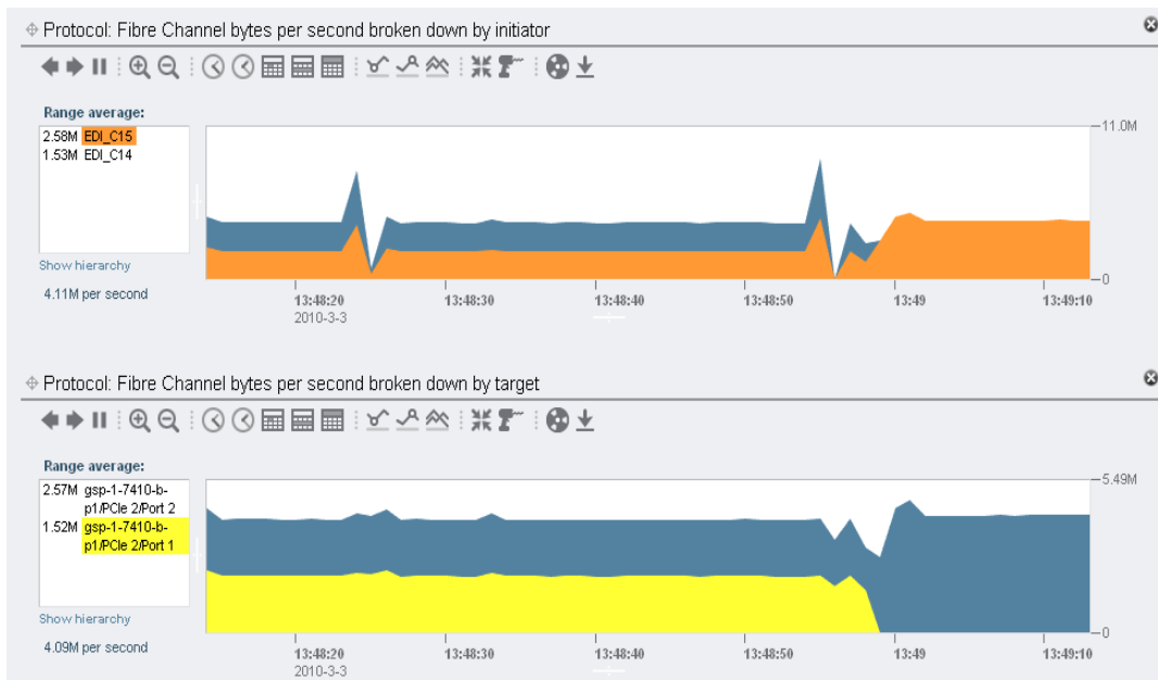
Figure 15. One FC Link failure
