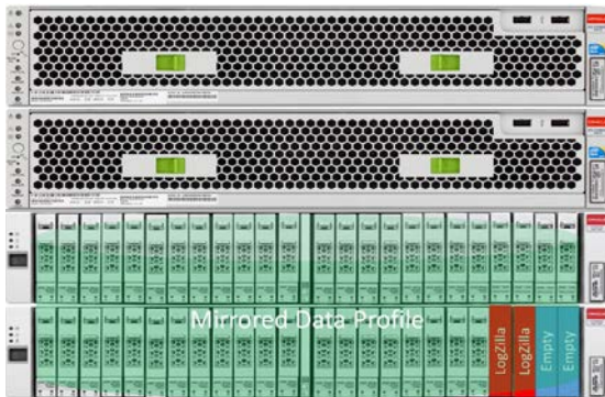
Figure 2. Oracle ZFS Storage Appliance – recommended storage layout for Oracle VM 3 performance environments
