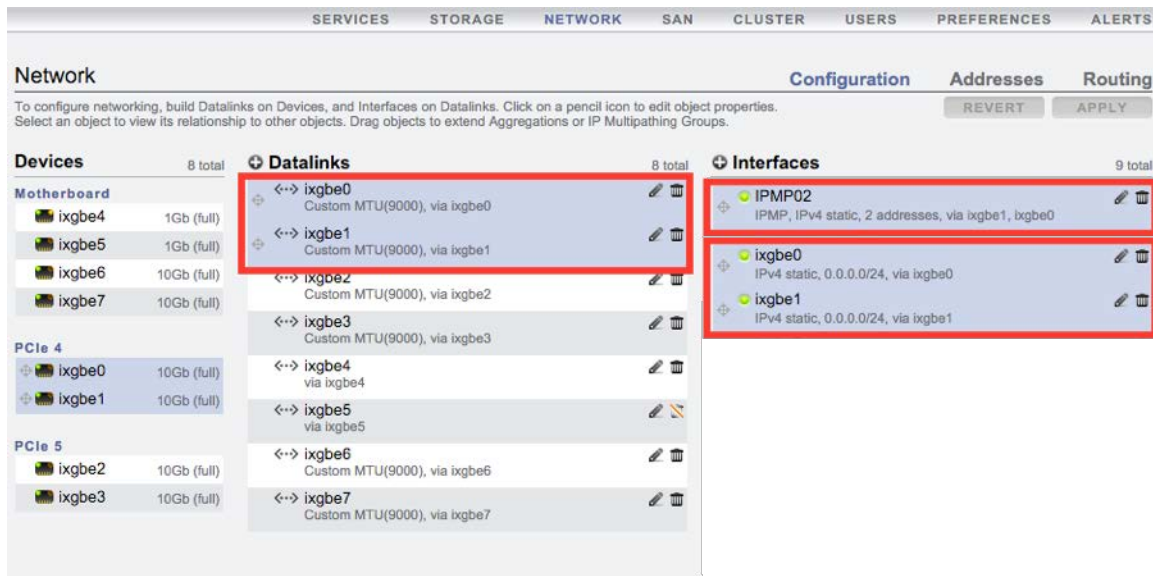
Figure 6. Example IPMP network configuration for Oracle ZFS Storage Appliance cluster head 2 and Oracle VM 3
