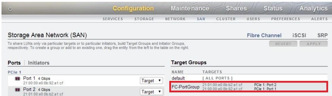
Figure 7. Completed FC target group in the Oracle ZFS Storage Appliance
