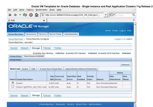
The OneCommand for Oracle VM build engine, Oracle RAC or ASM do not require that disks have identical names or ordering on all nodes, however, it might be easier for humans to deal with identical names and ordering. Therefore it is recommended to add disks in same order with same disk names to all VMs, e.g.; ASM1, ASM2, ASM3, ASM4, ASM5.
