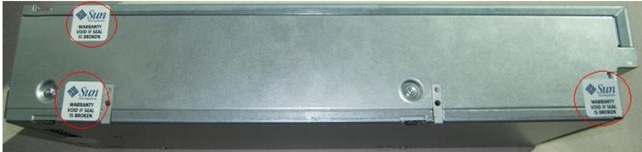
Figure 9: Tamper Evident Seals on Right Side
